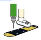
Drill 12MM diameter holes into the surface, through the existing holes of the placed units. The holes should be 120-140MM deep in order to accommodate the plastic shields that are 100MM long.
