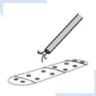
Make sure the holes are clear of dust and debris before installing the shields. After each hole is drilled, insert a plastic shield in order to keep the units from shifting.
