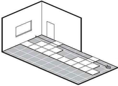
2. Loose lay the tiles (without adhesive) starting along the centrelines and following the arrows printed on the back of the tile staking special care to the alignment of joints and/or pattern.
