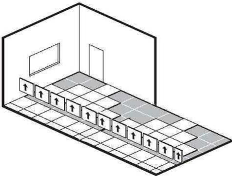
3. Check the uniformity of colour and the absence of defects. The perimeter tiles will require to be trimmed off to be ready for bonding.
