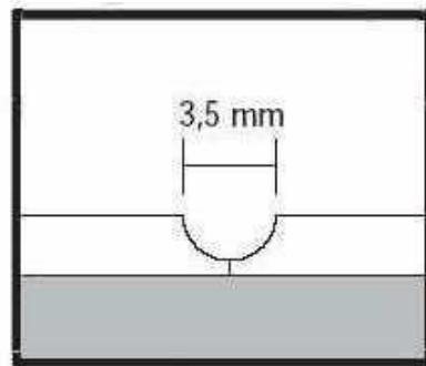
2. Place the sealing rod into the speed weld aperture, press the rod down into the groove and proceed at the right speed keeping the speed weld toe parallel to the rubber surface.
