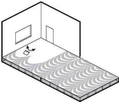
3. Lay the tiles starting along the centre lines and following the arrows printed on the back of the tiles taking special care to the alignment of joints. Cut the perimeter tiles to fit.
