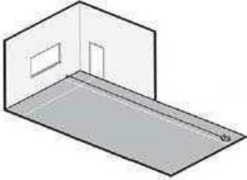
2. Loose lay the rolls (without adhesive) following the marked lines. Rolls must be laid with 3cm overlap along the adjoining edges. Check the uniformity of colour and the absence of defects.
