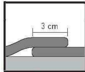
3. The loose laying is very important to check the colour uniformity and the absence of defects of the flooring. All claims will be accepted only if the flooring is not yet permanently bonded.
