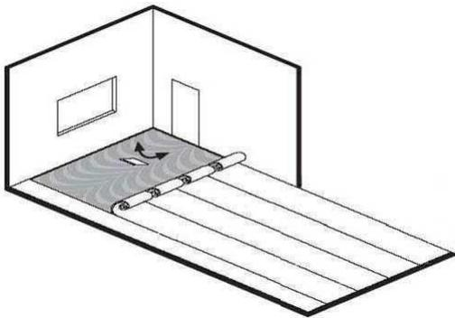
3. After the laying, the use of a floor roller is recommended to ensure a perfect contact with the substrate.
