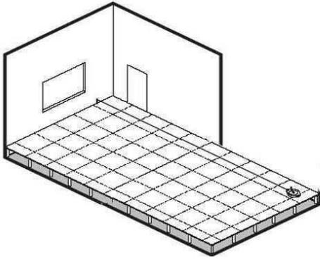
2. Apply the permanent tackifier with a notched trowel in accordance with the instruction of the manufacturer. Allow the adhesive to dry sufficiently.
