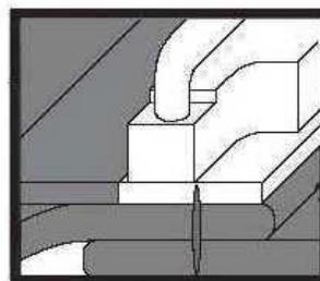
1. Fold back the sheet to just over half its length. Spread the adhesive using a notched trowel. Once the adhesive is ready to accept the flooring, roll the sheet back into place, taking care not to twist the roll or to trap air bubbles, which will eventually have to be expelled through massaging.
