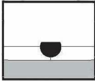
4. When the rod has cooled to room temperature the remaining excess should be trimmed using the spatula knife without the guide keeping a shallow angle between blade and floor to avoid "digging in". Attention: the colour of the rod cannot be exactly the same of the floor.
