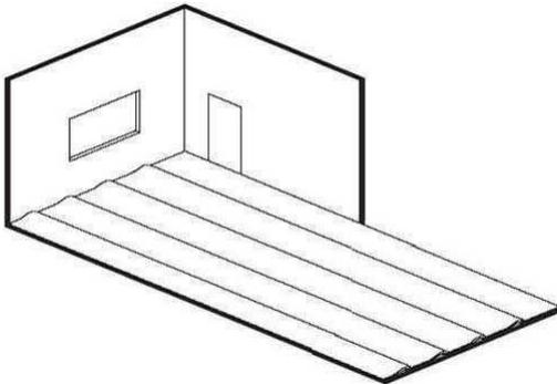
4. Perform the seam cutting along the sides and the heads of the rolls (the use of scribes and straight and hook bladed knives is advised to get better results).
