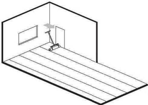
4. In case adhesive with long tackifying time are used, apply weights along the joints (bricks, sand bags, etc.).
