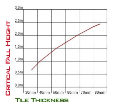
A special feature of Polymax safety tiles is the large hollow cone foot, and moulded base, which is designed to improve the critical fall height, and absorb much of the energy of a fall. This allows their use in a wide range of play area situations, and other leisure uses.
